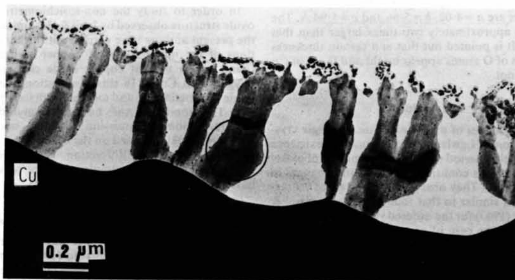
Fig. 1. Copper oxide film, formed on the surface of a thin copper crystal by heating at 770–820 K in a vacuum of 2–2.4 Pa for 2 min. Some parts of the oxide region have evaporated. The thickness of the film indicated by a circle is 100–200 Å.
